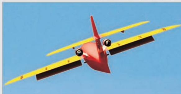
wing equipped with high-lift devices
